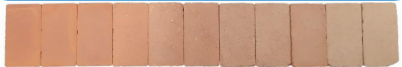
Image of a sample of each family of ceramics made from stone cutting sludge. From left to right, 0S10C, 1S0C, 2S8C, 3S7C, 4S6C, 5S5C, 6S4C, 7S3C, 8S2C, 9S2C, and 10S0C.
